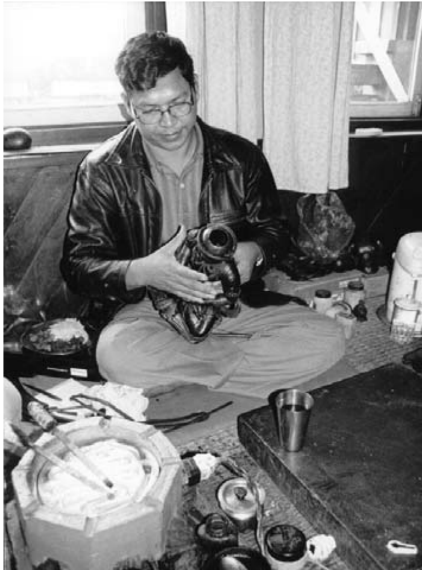
Plate 5.4 - Preparation of a wax model in a laboratory of a Patan Shakya family
