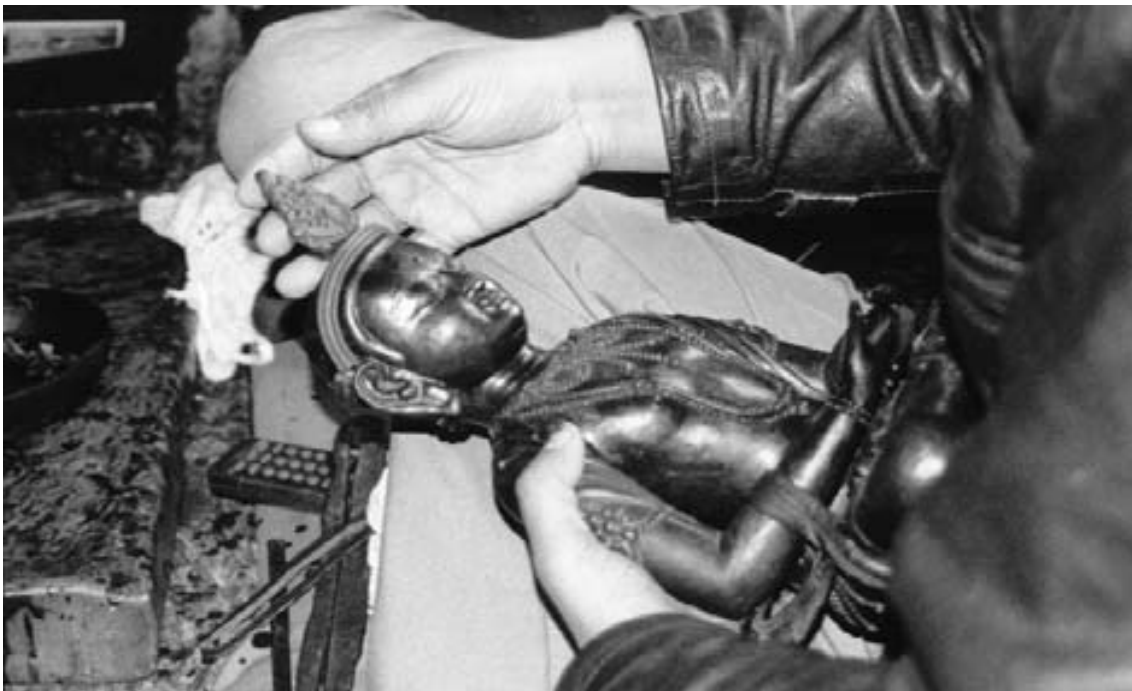
Plate 5.5 - Final touches being made to a wax model in a laboratory of a Patan Shakya family
