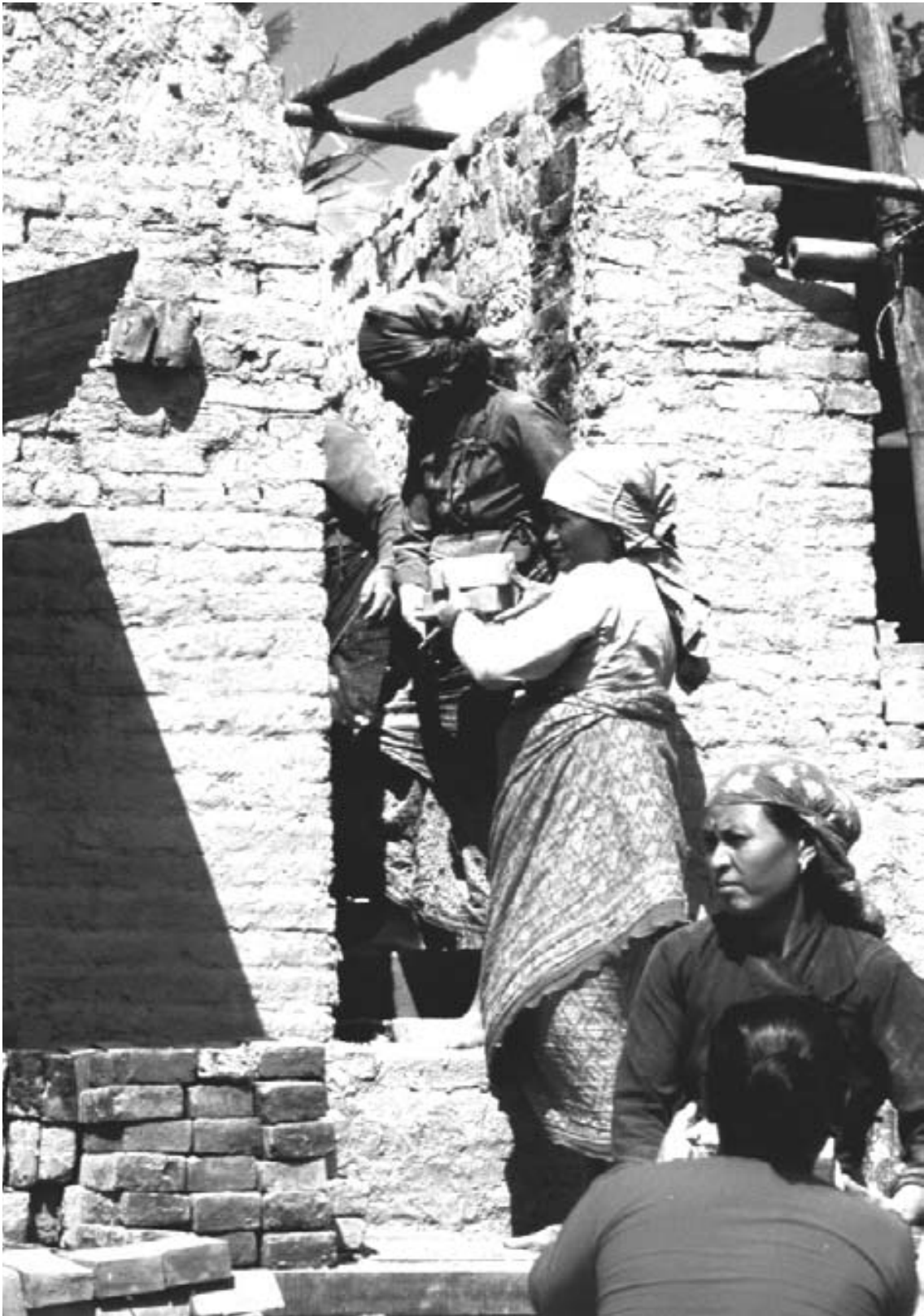
Plate 2.14 - Bricks are unloaded from an Intermittent kiln
