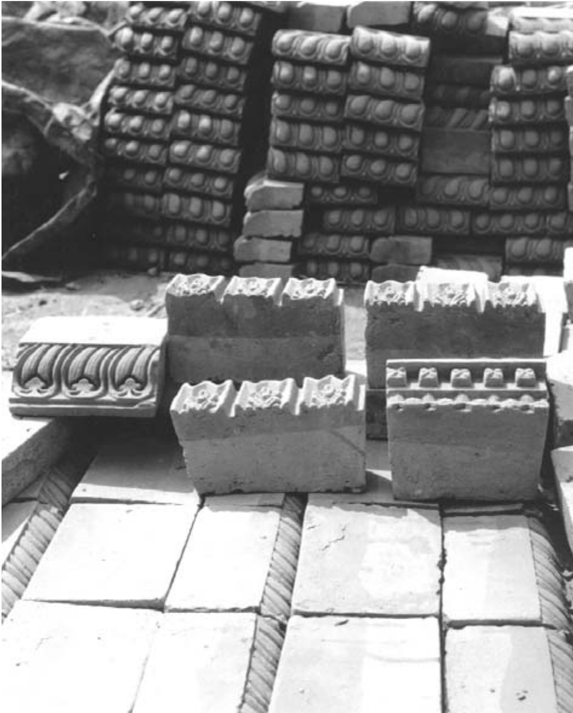
Plate 2.16 - Bricks used for frames and other decorative elements
