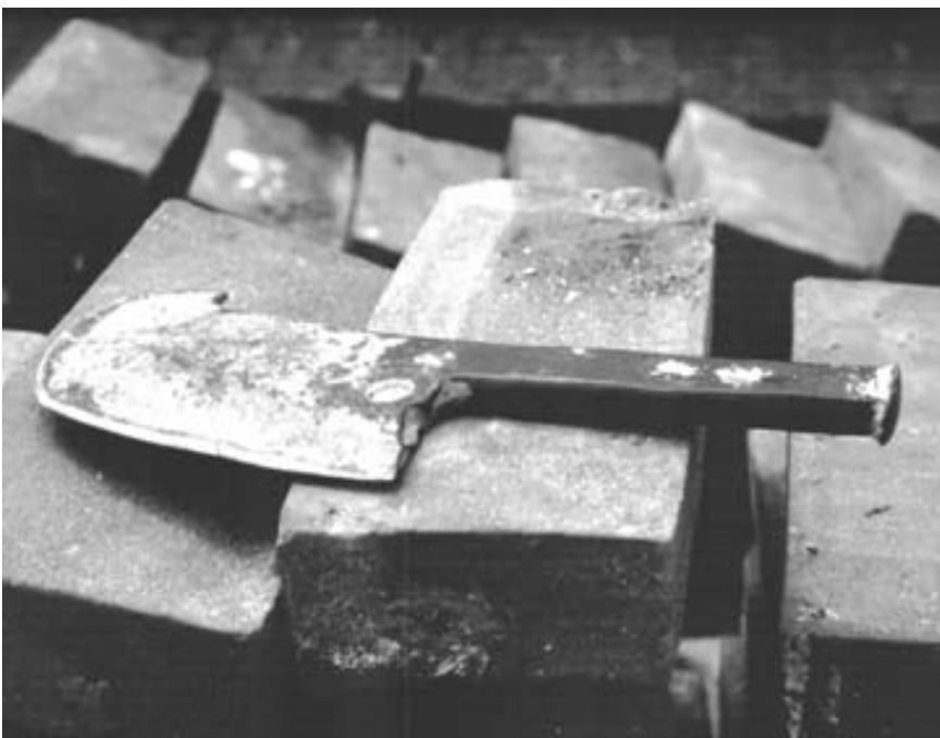
Plate 2.5 - Knife used for cutting bricks
