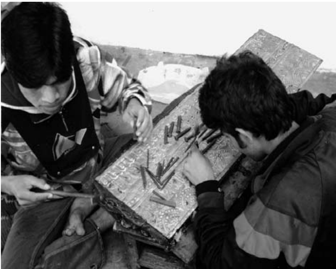
Plate 5.9 - Preparation of a prayer wheel using the repoussé technique
