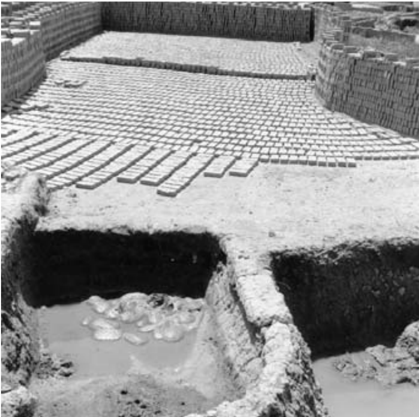
Plate 2.1 - A clay quarry with bricks drying in the open air
