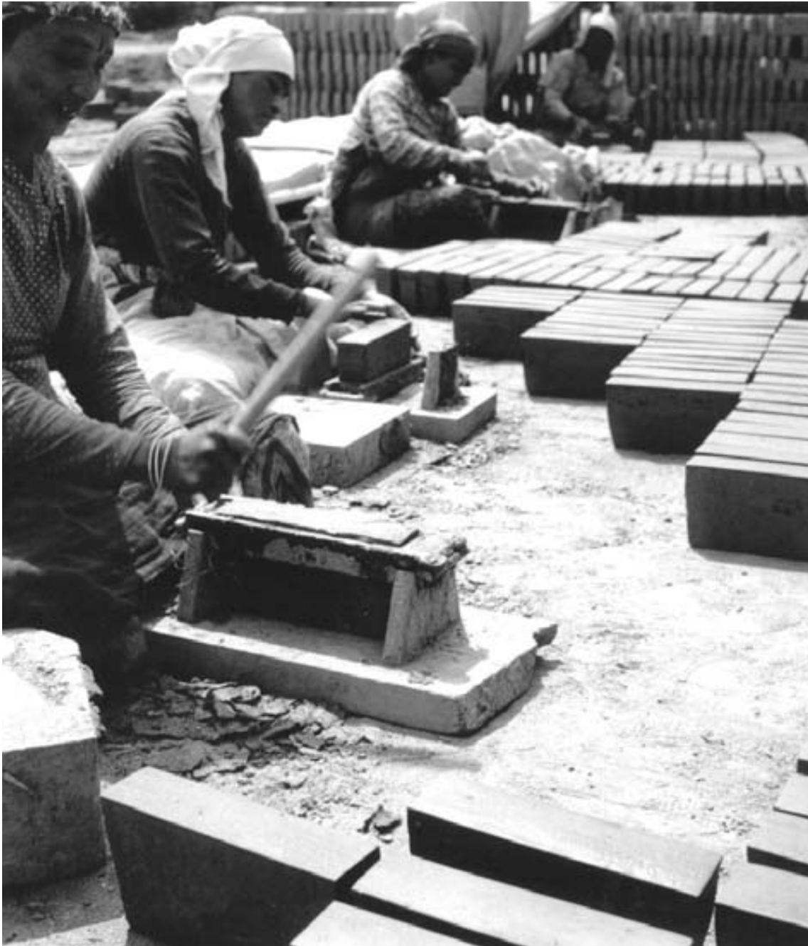
Plate 2.3 - Flattening of the fair-face of the daci appa with a mallet
