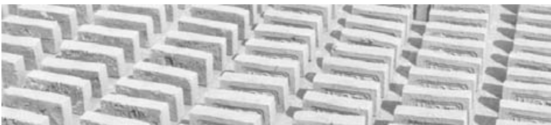
Plate 2.15 - Daci appa bricks dry in the open air
