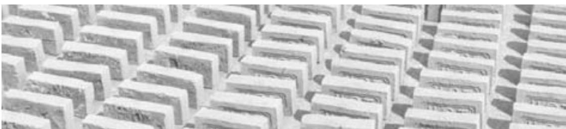
Plate 2.14 - Bricks are unloaded from an Intermittent kiln
