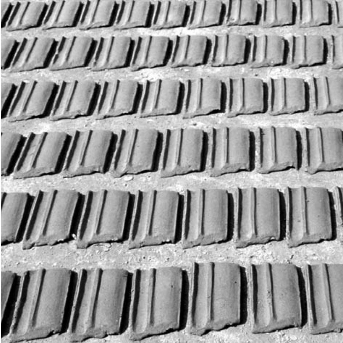
Plate 2.6 - Clay tiles dry in the open air
